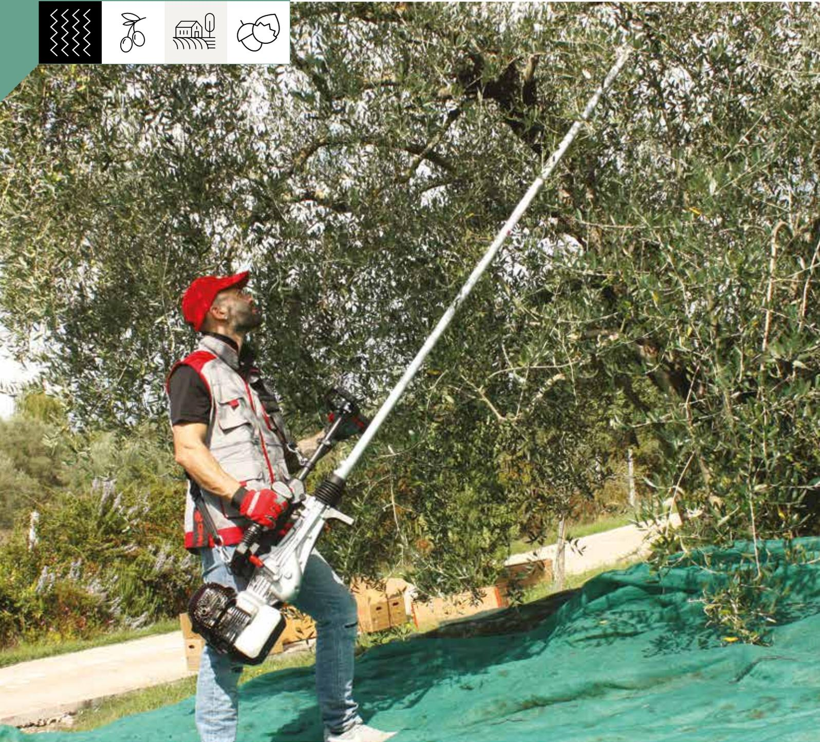
The **SC605** olive shaker for the harvesting of olives and other fruits is an ergonomic and light machine with features that are also suitable for professional use. The combination of ergonomic elements such as reduced weight, adjustable handles with anti-vibration, padded leg protection, combined with the powerful motor designed for olive shakers allow efficient and fast harvesting work.
